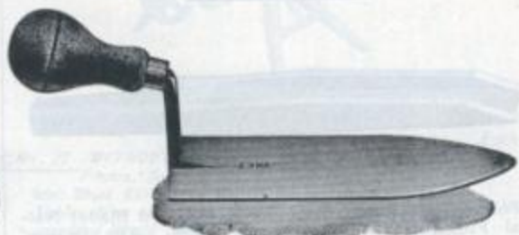
No. 2—Finishing Trowels.
